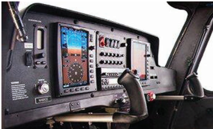
Figure 17-11. Stoke flight control with conventional engine controls.
