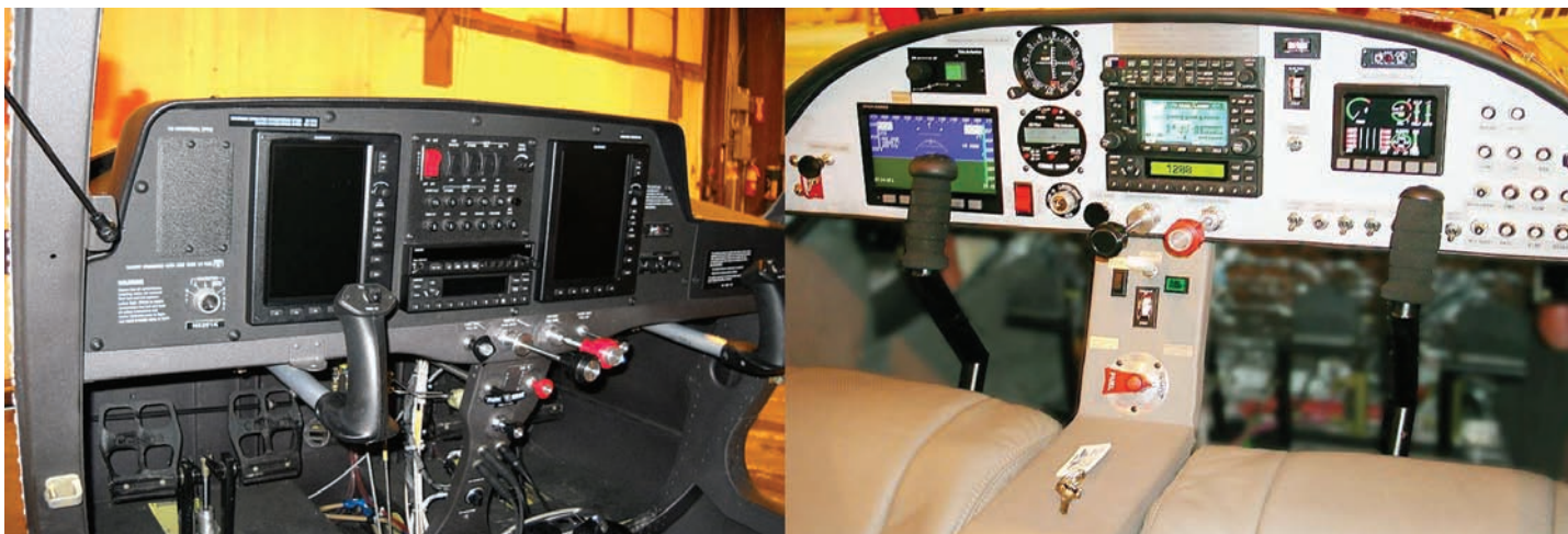
Figure 17-5. An electronic flight instrumentation system provides attitude, airspeed, altimeter, vertical speed, direction, moving map, navigation, terrain awareness, traffic, weather, and engine data all on one or two liquid crystal displays.
