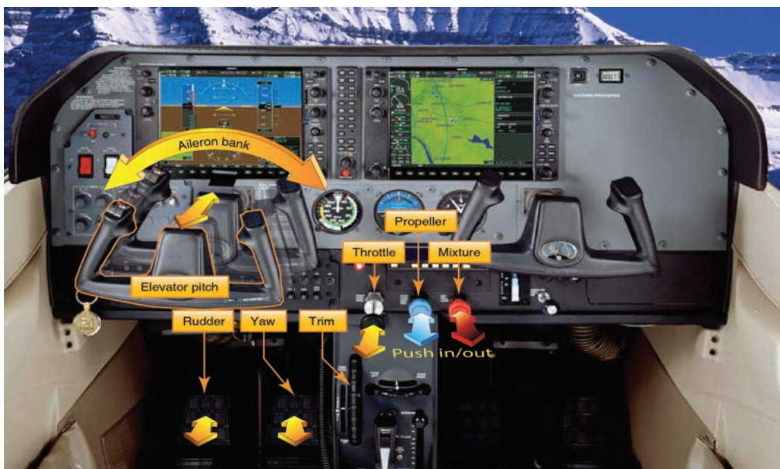
Figure 3-1. Basic flight controls and instrument panel.
