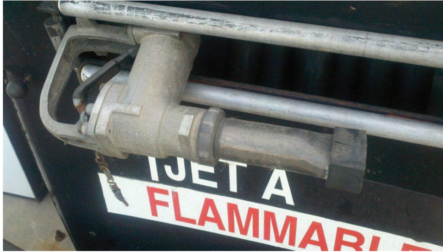
Figure 2-11. A jet fuel filler nozzle is flared at the end to prevent an inadvertent insertion into an AVGAS tank.
