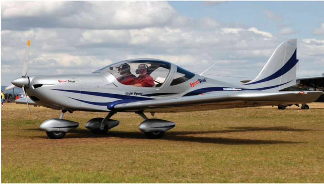
Figure 17-3. LSA can be constructed using both metal and composites.
