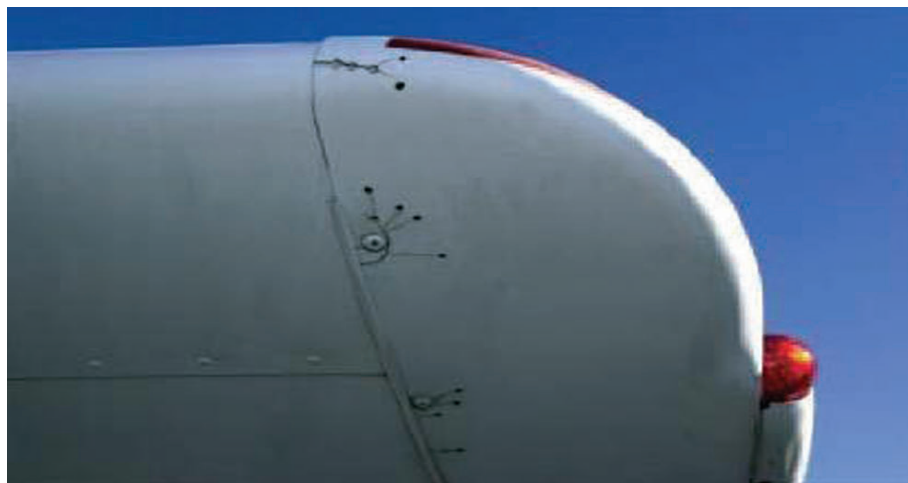
Figure 2-8. Cracks radiating from screw holes that have been stop-drilled to prevent crack progression.
