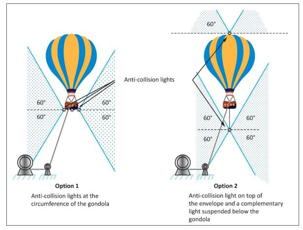
The horizontal 360° coverage requirement is applicable to a distance between 100 m and 3 700 m (2 NM). It is acceptable that the light from the anti-collision lights is not visible from positions closer than 100 m horizontally from the balloon.
