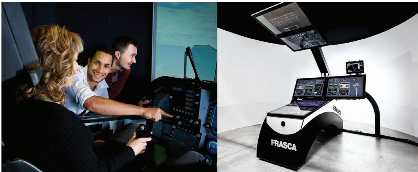
Figure 9-4. A level 4 FTD used for procedure training.
